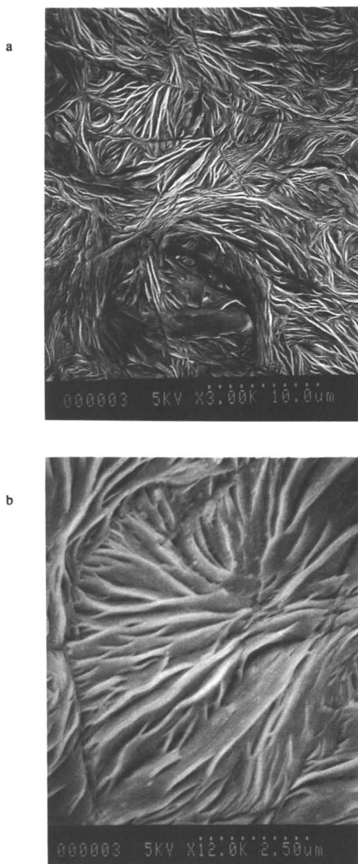
Figure 10. SEM Micrograph of etched s-PP spherulitic morphology. a. 2160X. b. 8640X.
